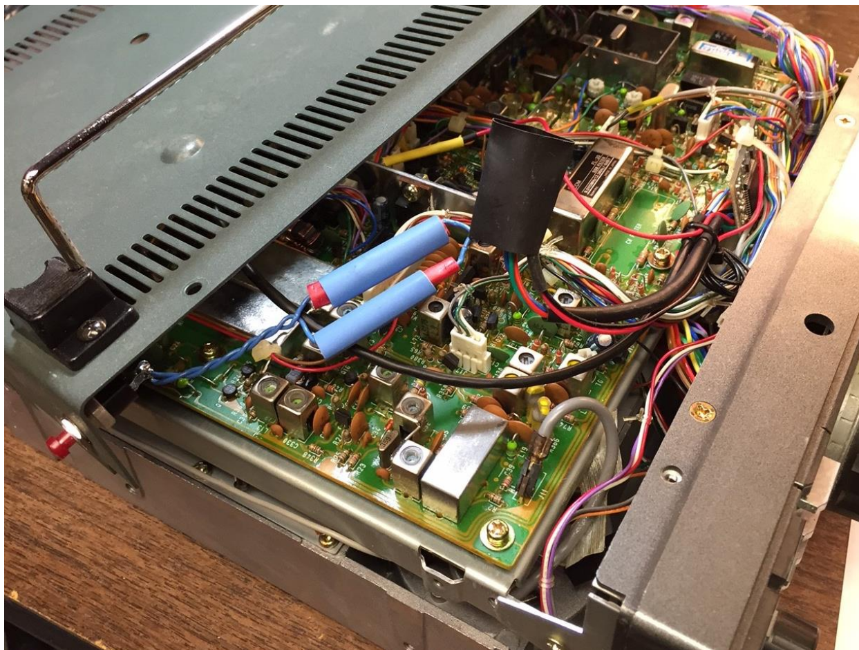
Figure 10. DSP board and push-button switch installed. The board is secured to the wiring bundle with a cable tie and a large piece of shrink wrap covers the DSP keyboard.
