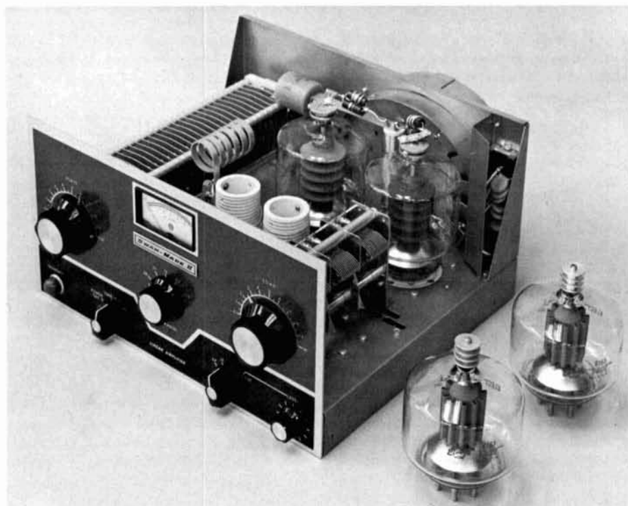
New Swan Mark II linear amplifier, designed to use either Eimac 3-400Z (foreground) or 3-500Z (installed in amplifier). The Swan incorporates zener bias to reduce zero-signal plate current of the 3-500Z tubes; bias may be switched out for the 3-400Z's.
