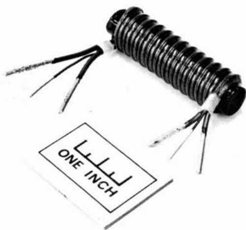
Filament choke for grounded-grid amplifier is wound on ferrite core, one-half inch in diameter and three inches long. The text explains how to build your own.
