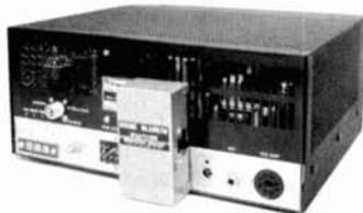
**TNB-250 shown installed on Swan 250 by means of the pre-punched accessory holes.**
