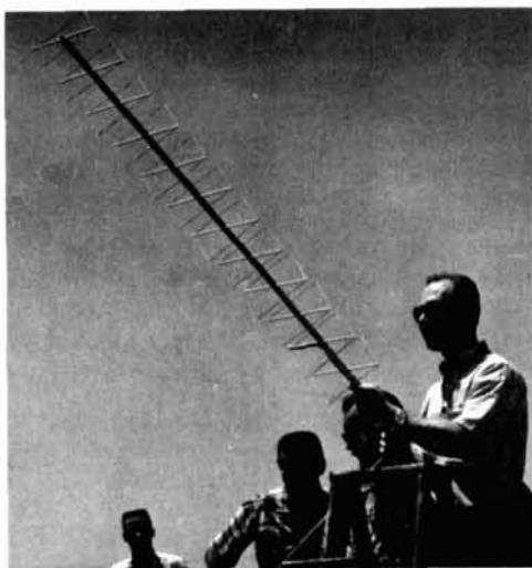
K6MYC's 12-element 432-MHz quad gave 7.9 dB.
