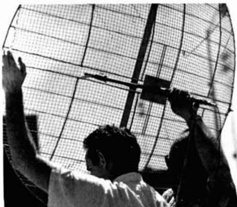
WA6KKK and WB6MGZ aim 18.6-dB 1296-MHz dish.
