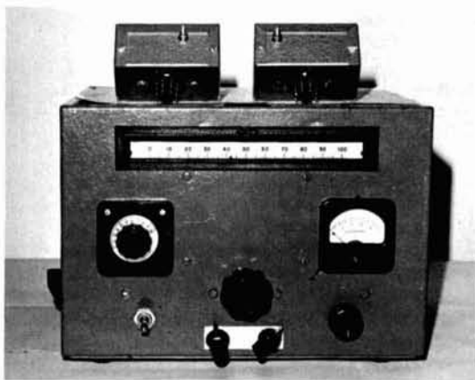
The 80- and 40-meter transceiver. Plug-in exciter units are on top.
