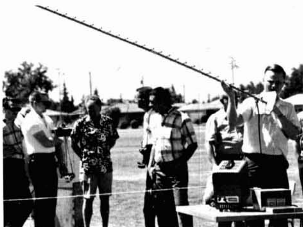
K7ICW's 30-element Yagi for 1296 MHz yielded -2.5 dB!
