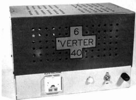
The ventilated cover improves appearance and provides essential shielding and protection from accidental contact with the high voltage.
