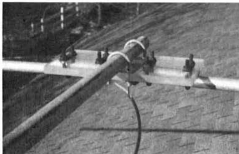
fig. 1. Basic construction of a rotatable dipole element showing the use of U-bolts and a scrap piece of plastic.
