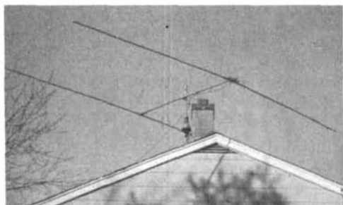
fig. 3. Simple arrangement for adding a reflector to a 15-meter dipole.
