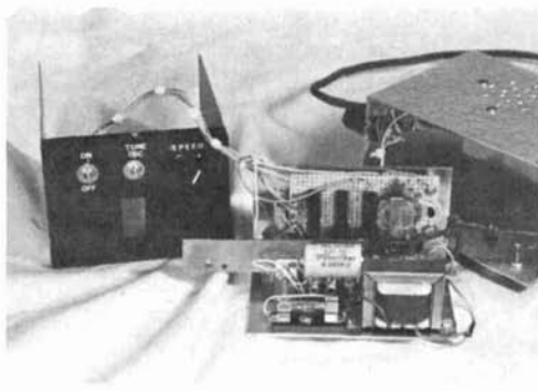
Construction of the cosmos keyer. Circuit board, keying mechanism and power supply are on center chassis. Speed control and switches are mounted on front panel, left.
