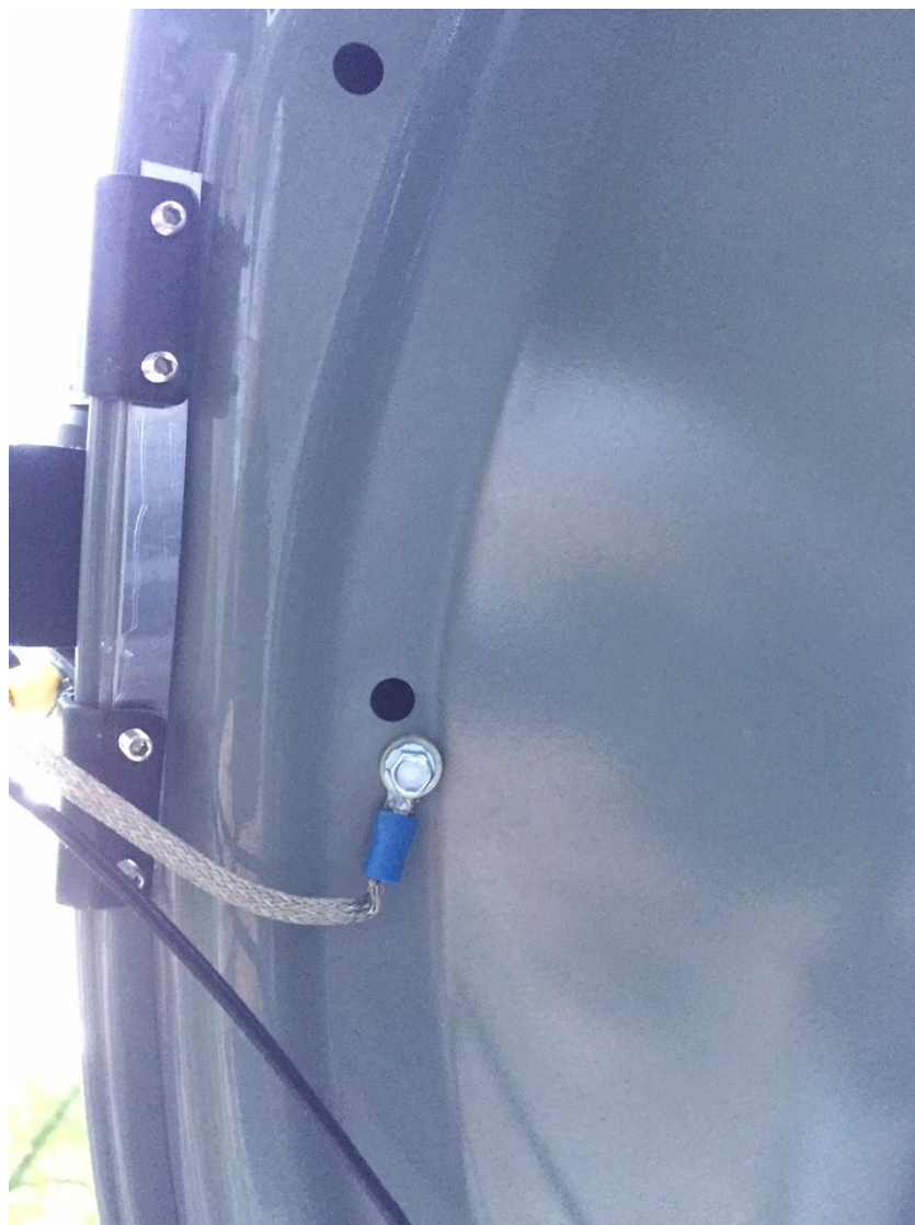
Figure 3. Underside of the hood showing the ground connection
