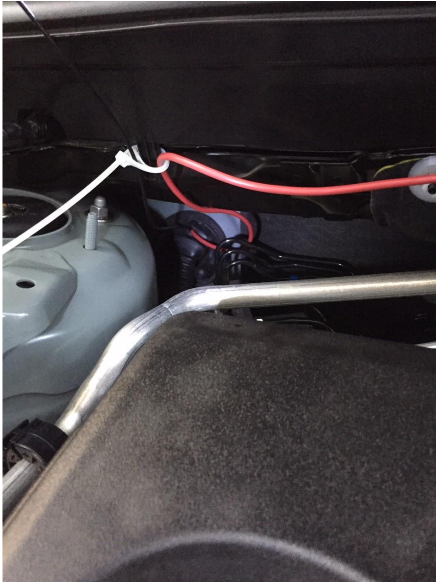
Figure 4. Cables routed through the grommet
