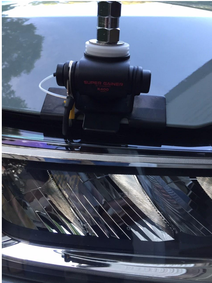
Figure 2. Detail of mount on the non-curved section of the hood
